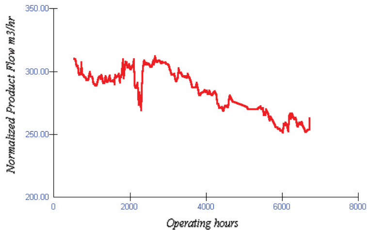
Fig. 4. ASTM-normalized flux decline trend — seawater RO plant.
